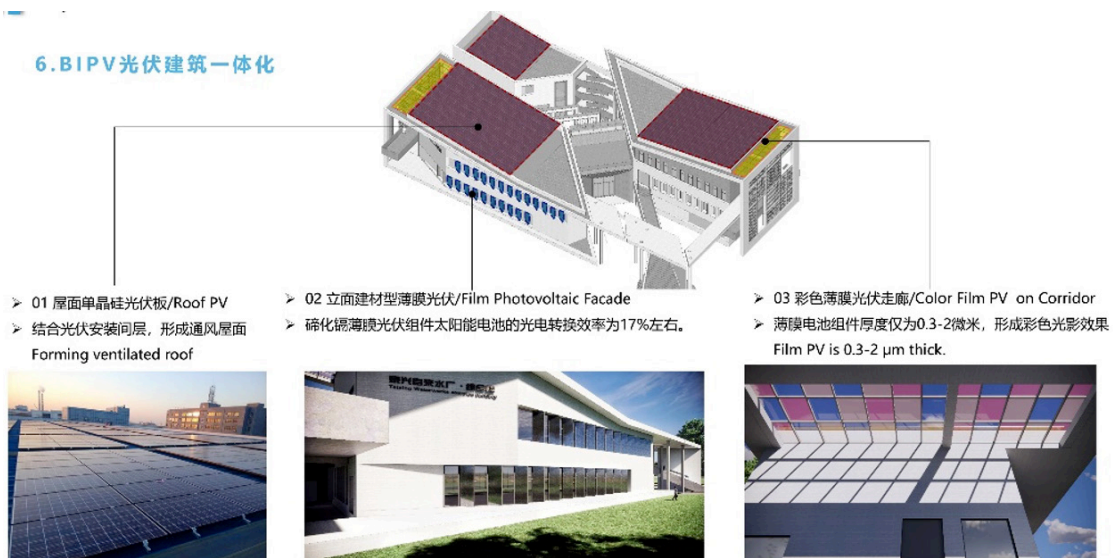
Figure 4: Building-integrated photovoltaics (BIPV) on Façade and PV on the roof
