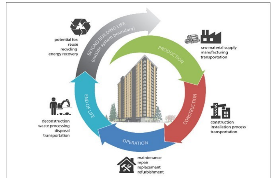
Figure 1: Understanding the whole life-cycle of buildings with the emission stages up- and downstream. Source: Archdaily.com
