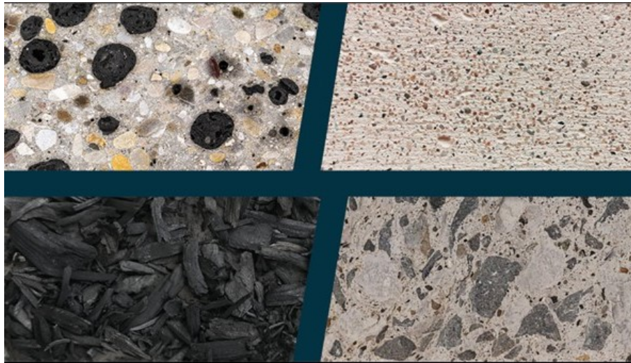
Figure 27: Biochar added to concrete; source: beyond zero/Empa
