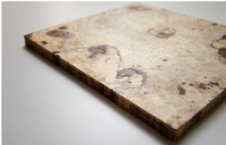
Figure 26: Actual research for building materials: «Mycelium-Bound Composite», a project by Future City Laboratory, ETH Zurich-Singapore; source: ETHZ
