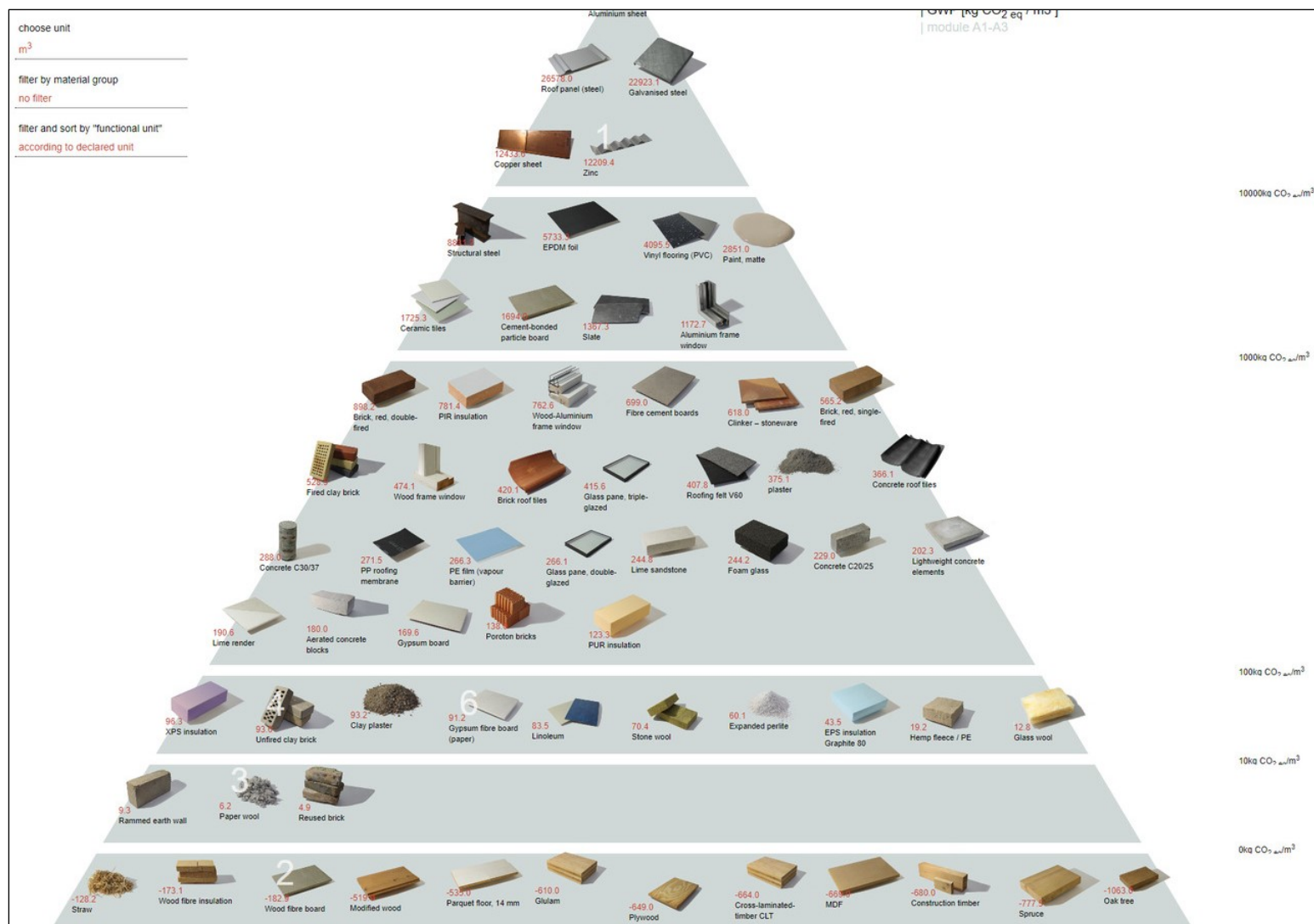
Figure 24: The Construction Material Pyramid from the Royal Danish Academy makes it possible to compare Carbon footprints between different categories of materials or between material types within the same category. It also makes it possible to view different kinds of environmental impacts across the different materials. Source: www.materialepyramiden.dk .
