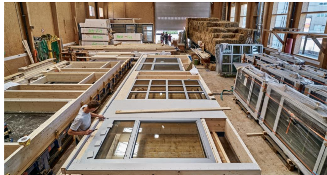
Suggestion 4: Wooden Facade with straw insulation
