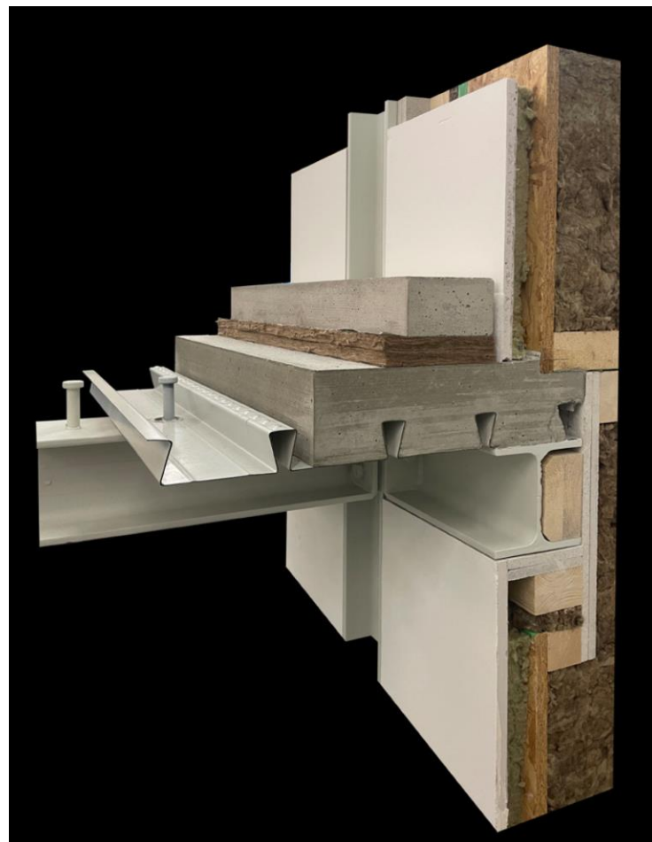
Herbstweg: connection steel frame wooden facade.钢框架与木质外立面的连接
