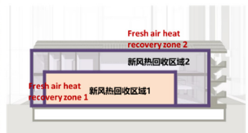
Figure 11. Zero carbon strategy – Active technology “fresh air heat recovery”, Beijing Demo Project of Sino-Swiss ZEB cooperation project - Gongchen Community Center of Fangshan District in Beijing. Graphics created by SUP and ZEB consulting Team of CABR.
