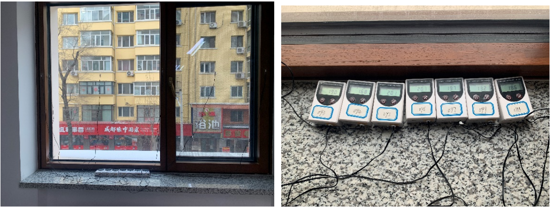
Figure 3: Temperature Sensors Installed to Monitor Temperatures at Different Points
